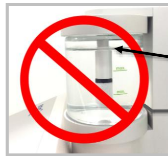
Fig. 5.2: Incorrect water levels (not between min and max)
