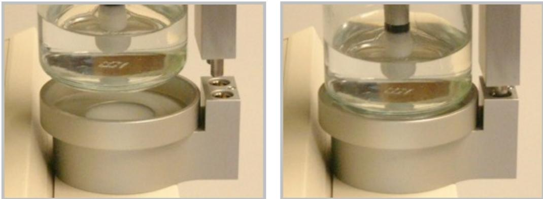
**Figure 5.3: Inserting humidifier into device**
