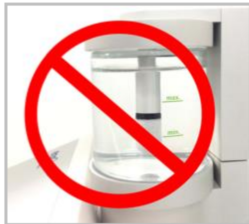
Figure 5.2: Incorrect water levels
