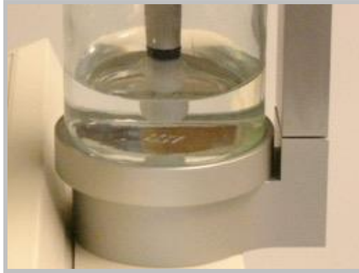
Figure 5.4: Correct insertion of humidifier
